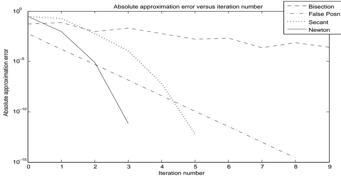
In particular, the trend for the Method of False Position is almost perfectly *linear*, while the trend for Newton's Method is almost precisely a *quadratic* curve.
