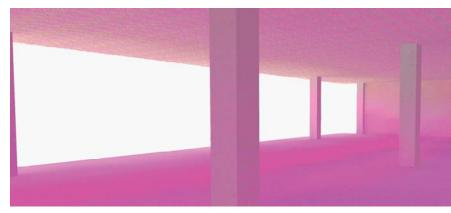
Digital model analysis of how natural daylighting penetrates into the 2nd floor studio space.
