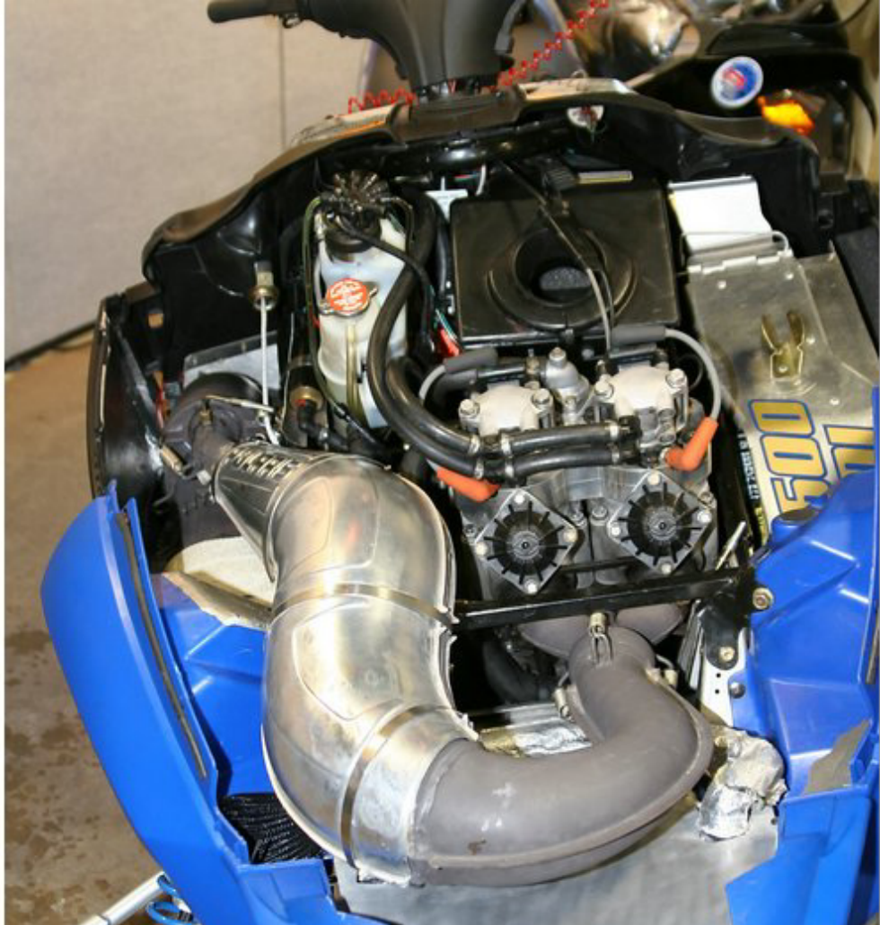
Figure 42: The final design of the naturally aspirated UI GDI engine [33].
