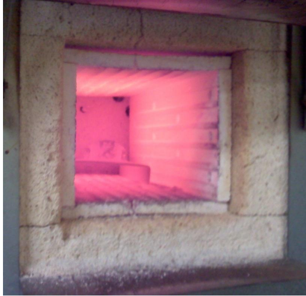
Figure 19: SCT Engine – Valve Annealing Process in Oven
