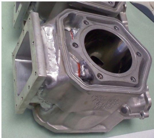
Figure 13: Cylinder Showing Permanent Insert, Welding and RTV Junction.
