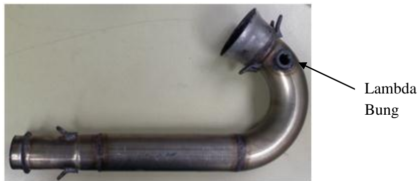
Figure 16: SCT Engine – Mid-Pipe
