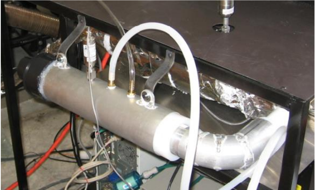
Figure 17: Tunnel body with transducer and sampling lines
