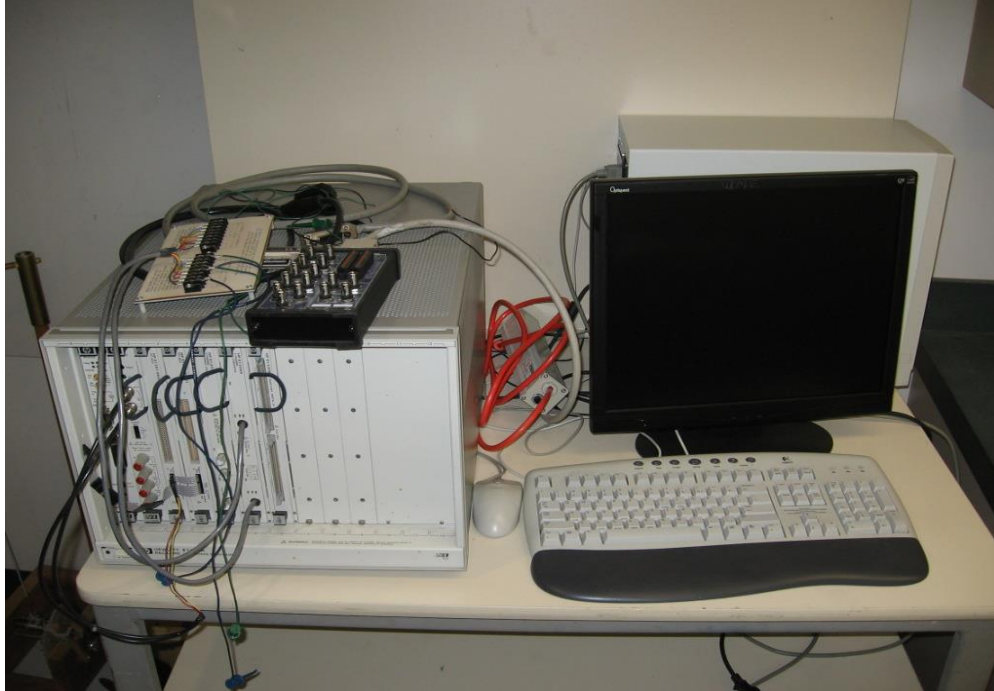
Figure 10: Hewlett Packard VXI Data acquisition unit
