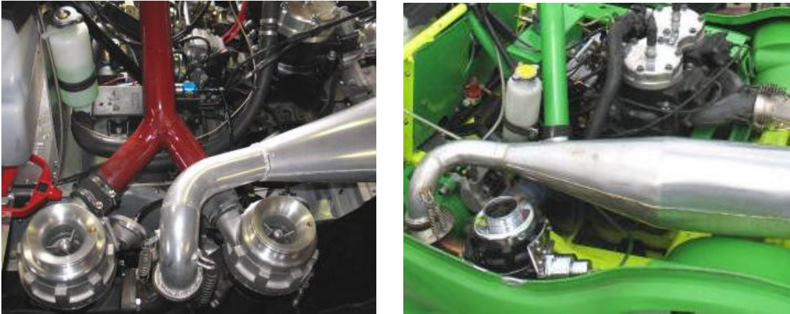
Figure 15: Aftermarket turbochargers installed on two-stroke snowmobile engines.
