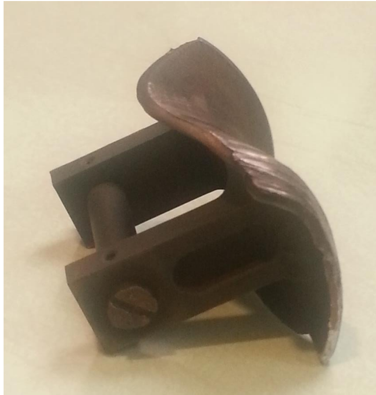
Figure 32: Mag Side Valve After Failure
