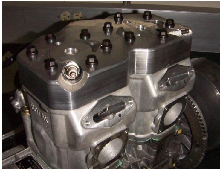
Figure 6: The University of Idaho GDI Cylinder Head
