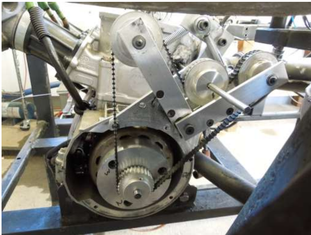
Figure 20: Manufactured prototype of the third belt drive design
