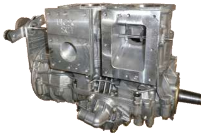
Figure 16: PR-SCT engine with one insert removed
