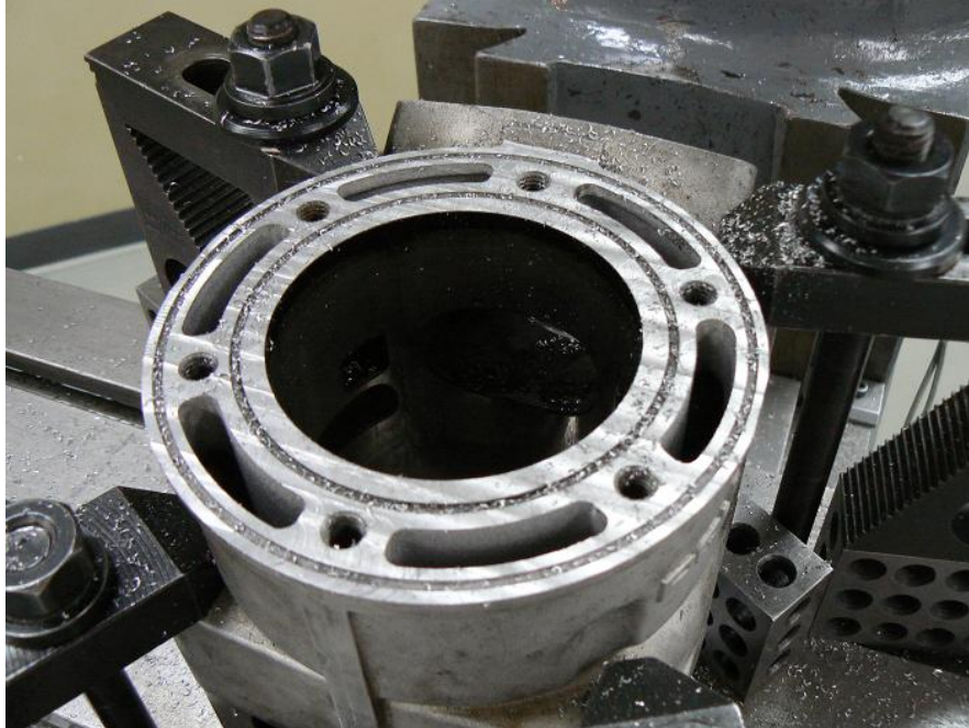
Figure 25: Cylinder machining finished.
