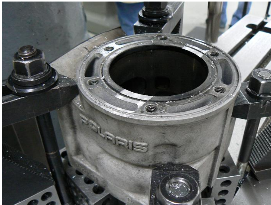
Figure 24: Cylinder machining in progress.
