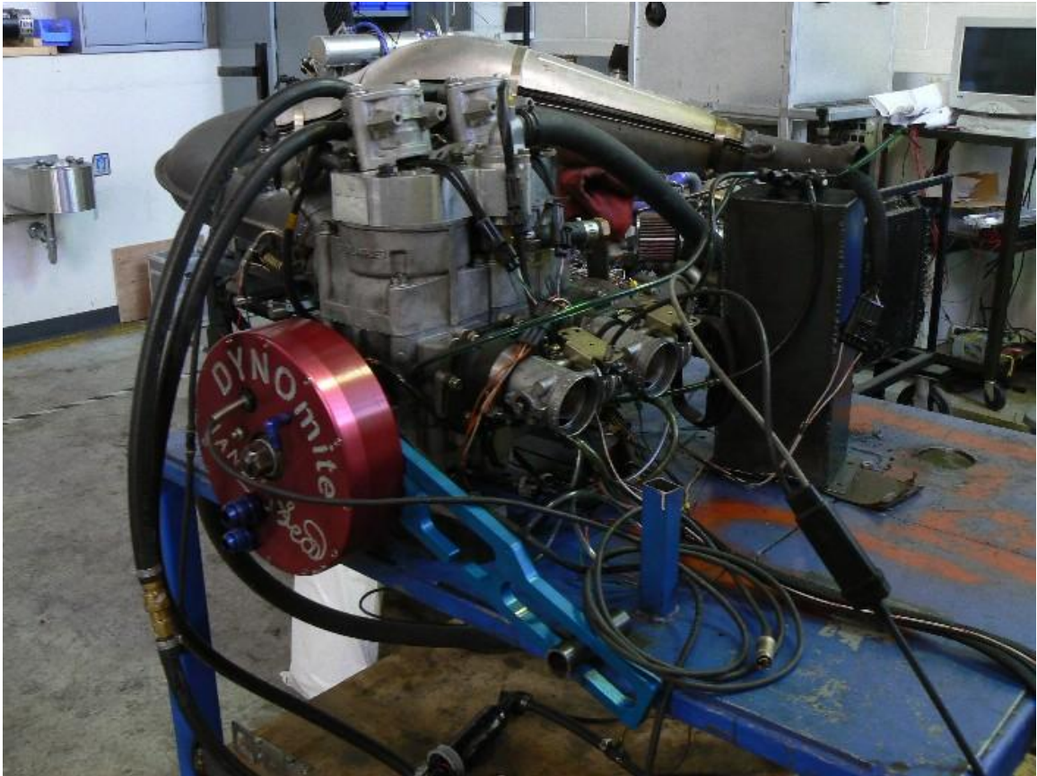
Figure 26: Dynamometer head attachment to the crankshaft.
