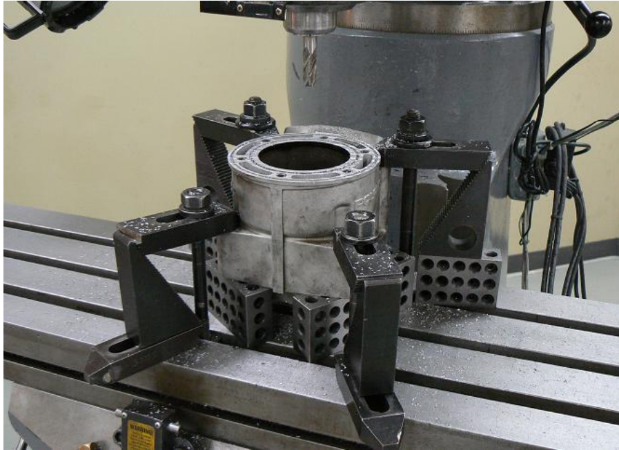
Figure 23: Equipment setup for machining cylinders.
