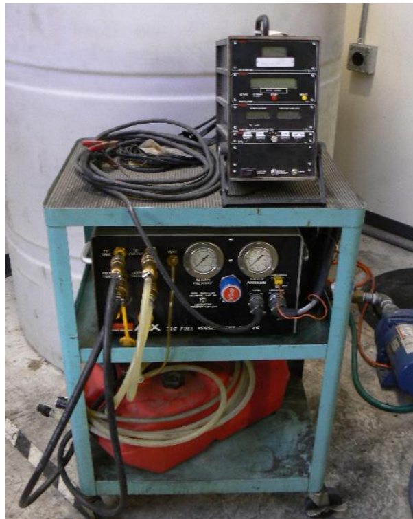
Figure 28: Fuel metering and display units.
