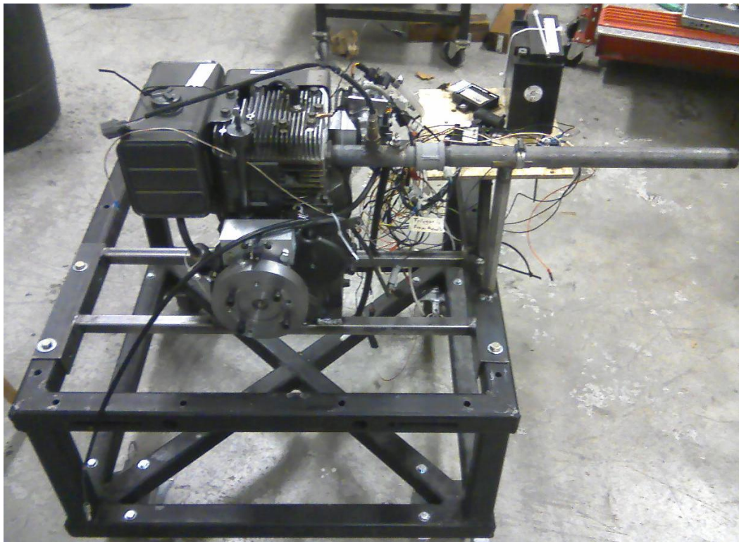
Figure 23 Engine on Test Stand
