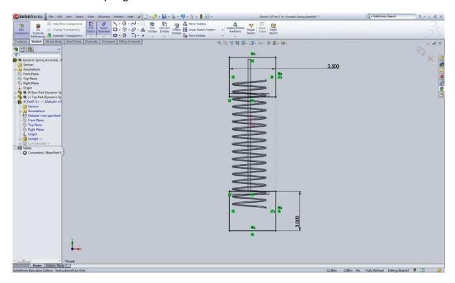
After cutting it you can exit the "edit component" by clicking on the "edit component" button again. Save it, it will ask if you want to save the new component, the spring, internally or externally, choose externally and specify a file path for your part. Once this is done you should be able to move the top disk of the assembly, hit rebuild and the spring will jump to where you moved the disk to. In an animation, the spring should move fluidly with your disk.
