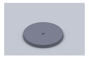
After these two parts are created, put them together in an assembly. Mating only the hole of the top part to the hole of the bottom as shown.
