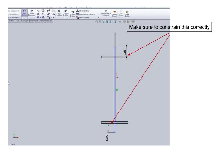
After constraining the sketch properly, the one inch dimensions are arbitrary, they can be anything you want them to be, create a new sketch on the front plane consisting of the cross section of your spring, in this case a small circle. Give it a horizontal relation with the end of the line that you made in the last sketch as well as a dimension showing how far away from the line it is.
