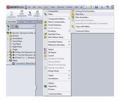
Once you have the new component in the design tree, you can select it in the design tree and then click on the "edit component" button at the top left of the screen under the "assembly" tab
