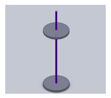
Once in the assembly with only one mate, add a new part through the "insert" drop down menu.
