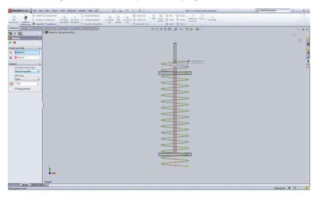
Next, create a new sketch on the front plane to cut the excess spring off of your creation. Create a shape to cut off the excess spring, and then use the "extruded cut" feature to cut the spring.
