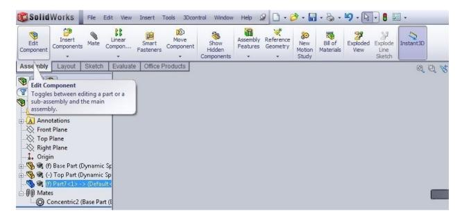
Once in, create a sketch on the front plane. Make one line constrained to the top/bottom of the disk pieces as shown in the picture below.
