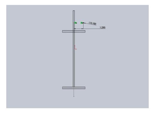
After making this sketch, click on "Swept Boss/Base" under the features tab. Use the circle as the profile and the line as the path. Under options in the sweep feature, pick twist along path as the orientation/twist type and define by: turns, pick the number of turns, click the green check, and now you have a spring.
