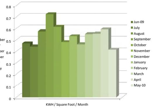
compared to other buildings on the University of Idaho campus. After obtaining monthly readings from the 07-08 and 09-10 school years (readings from June to May), the buildings overall EUI was calculated. AAN's EUI for 07-08 was 202, and for 09-10 it was 164. When compared to the University of Idaho average of 166, AAN scores slightly better than the average campus building.
