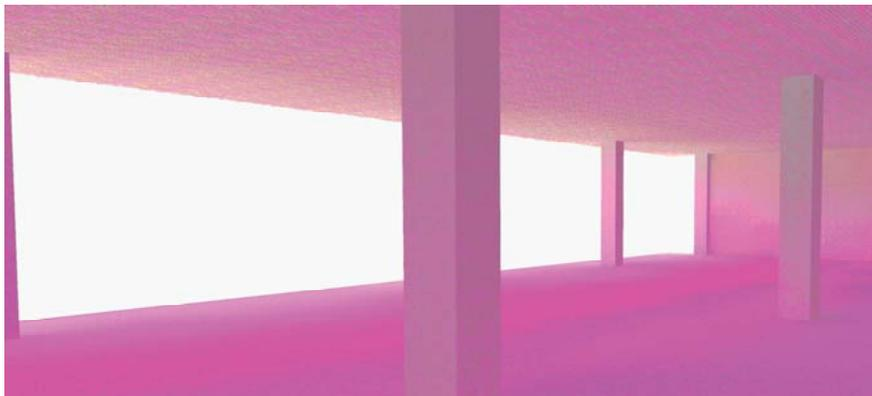
Digital model analysis of how natural daylighting penetrates into the 2nd floor studio space.
