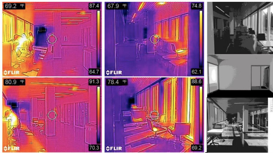
Figure 6: Infrared Camera and Glare Analysis: glare present.
