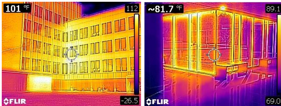
Figure 4: Late Afternoon Infrared Images of Glare: external (south- and west-facing curtain walls) and internal (study space along those walls).
