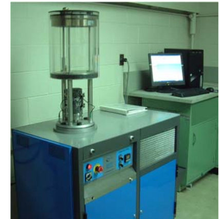
E* Testing using SPT Machine
