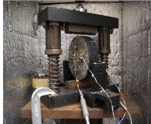
Indirect Tensile Tests Loading Frame and Specimen with LVDTs
