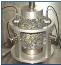
Arizona State University [F052] V1.09 Static Creep/Flow Time Strength Test
