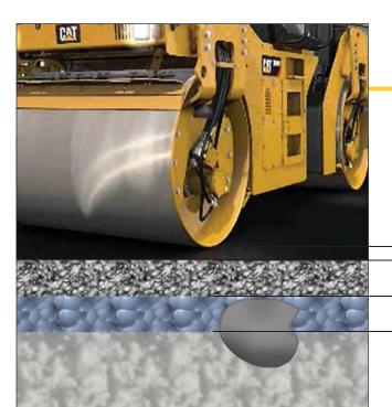
Accelerometer based technology measures deeper than the freshly laid lift of asphalt.
