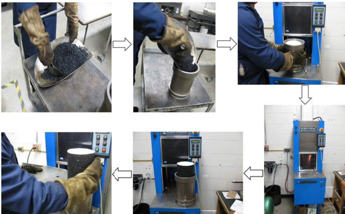
Figure 27. Sample Preparation and Compaction
