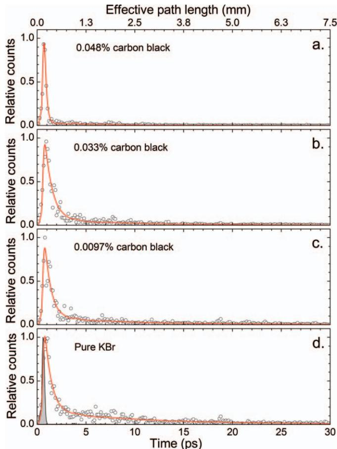
Fig. 3. Time-resolved data (circles) with bi-exponential fits (red curves). The gray shaded curve in the lower graph is the instrument response function. Plots (a), (b), (c), and (d) correspond to varying concentrations (weight percent) of carbon black; 0.048%, 0.033%, 0.0097%, and pure KBr, respectively.
