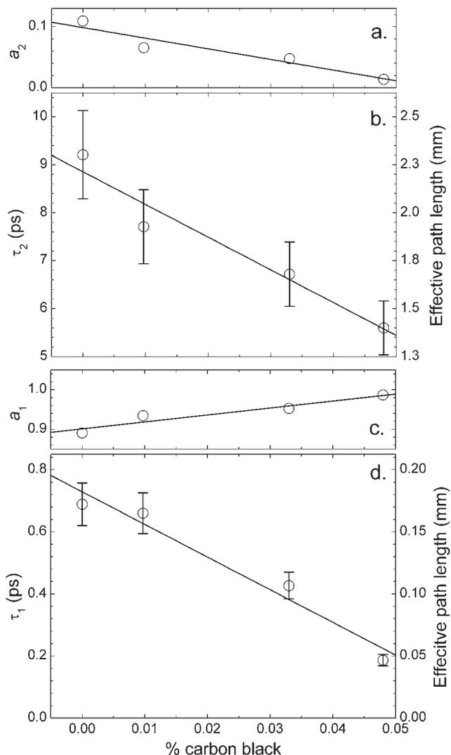
FIG. 4. Parameters from the bi-exponential fits. The slow time constant  $\tau_2$  and its amplitude  $a_2$  are shown in plots (b) and (a), respectively. The fast time constant  $\tau_1$  and its amplitude  $a_1$  are shown in plots (d) and (c), respectively.
