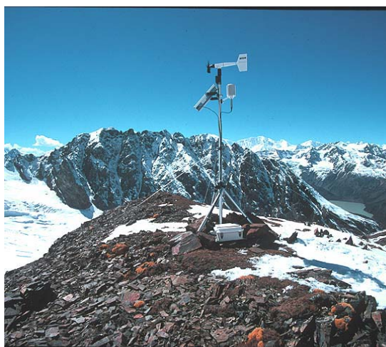
Figure 2.7. ‘Campbell Scientific’ automatic weather station established at 5,800 m, 2 km northeast from proposed drilling site at Zuoqiupu Glacier snow-firn area. Photo by D. Joswiak
