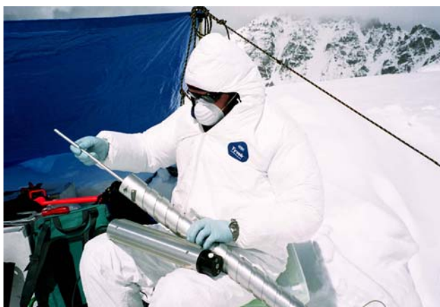
Figure 2.6. ‘Mini-Felix’ sun powered electro-mechanical drill. Drill barrel cleaning after each run. Zuoqiupu Glacier, 6,120 m a.s.l proposed deep drilling site. Photo by V. Aizen
