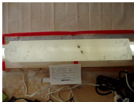
Figure 1.13. Loosed stones close to the bottom at 169.6 m depth.
