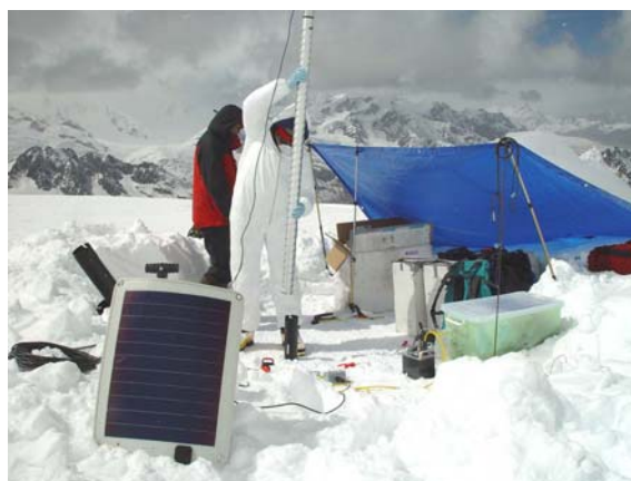
Figure 2.8. ‘Mini-Felix’ sun powered electro-mechanical drill. Zuoqiupu Glacier, 6,120 m a.s.l proposed deep drilling site. Photo by V. Aizen
