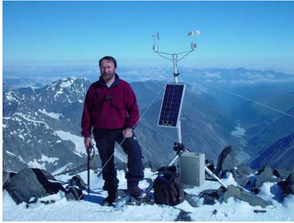
Figure 1.5. Automatic weather station installed at 4100 m a.s.l., 0.5 km north from the drilling site. July 2002, photo by V. Aizen
