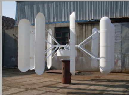
Vertical Axis Wind Turbine (VAWT)
