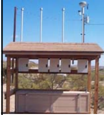
The IMPROVE Modular Aerosol Sampler which, measure fine and total aerosol mass. The sampler was developed and refined by the IMPROVE program, and has been in operation since 1987.
