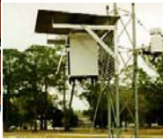
The Optec NGN-2 integrating nephelometer , which estimates the atm. scattering coefficient by directly measuring light scattered by aerosols and gases in a sampled air volume.
