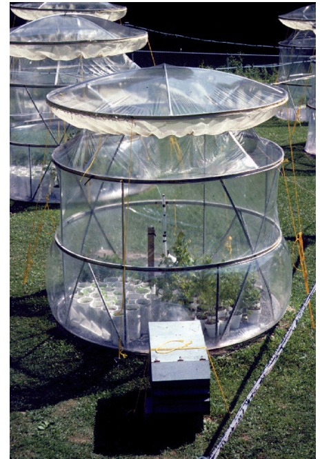
Researchers use fumigation chambers such as these to expose different plant species to varying amounts of ozone pollution in order to document the type of injury or damage that occurs from different levels of exposure. This type of experiment was used to determine which types of plants were being affected by ozone pollution at Great Smoky Mountains National Park. Nearly 100 different species of plants have shown ozone-like injury symptoms.
