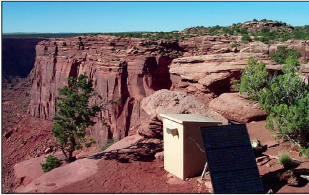
Transmissometer transmitter component at Canyonlands National Park, Utah. Transmissometers measure atmospheric extinction (total visibility reduction due to particles and gases). Measurements can be converted to visual range.
