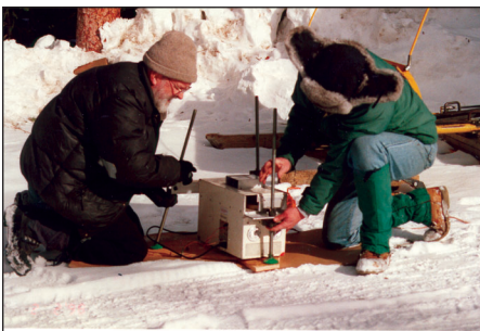
University of Denver researchers measure snowmobile emissions at Yellowstone National Park. Snowmobiles emit significant amounts of carbon monoxide and hydrocarbons during the 3 months that they are allowed in the park. Between 60,000 and 70,000 snowmobiles enter the park each winter.
