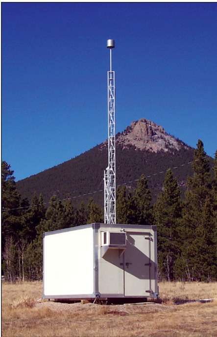
Measurements obtained from this air quality monitoring station at Rocky Mountain National Park, Colorado, and other stations located in national parks are used to estimate dry deposition levels of acidic air pollutants to park ecosystems.
