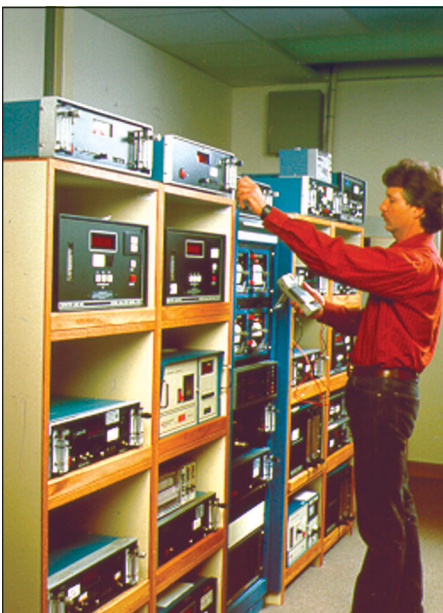
Air quality instrumentation are calibrated and serviced in a laboratory prior to deployment for special studies or routine monitoring.
