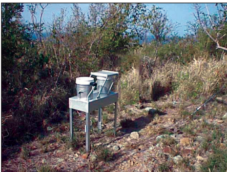
Precipitation collectors such as this one at Virgin Islands National Park are used at 42 park locations to measure the chemical composition of rain.
