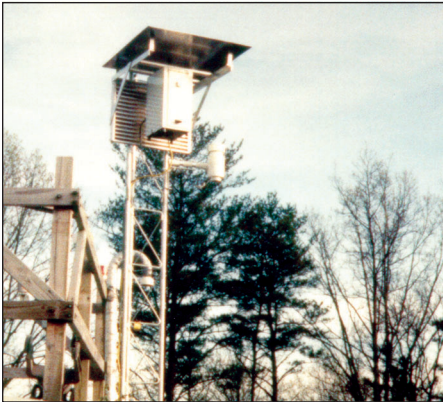
Nephelometer monitoring system at Great Smoky Mountains National Park, Tennessee/North Carolina. Nephelometers measure the amount of light scattering, and hence visibility reduction, caused by fine particles, and are used routinely in many national parks.
