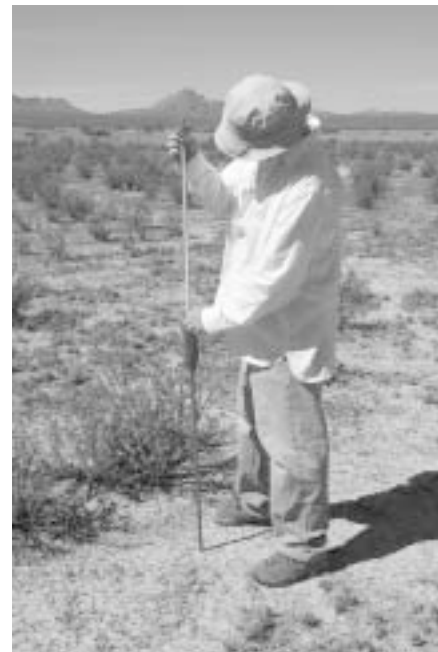
Figure 7.2. Hammer height is the distance from the hammer to the strike plate.
