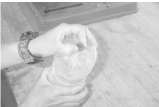
Figure A.9. Drill hole in bottom of wide-mouthed, 32 oz soda bottle and insert stopper.
