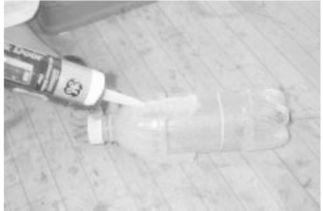
Figure A.10. Apply three 10 cm silicone beads from top of bottle to mid-section.
