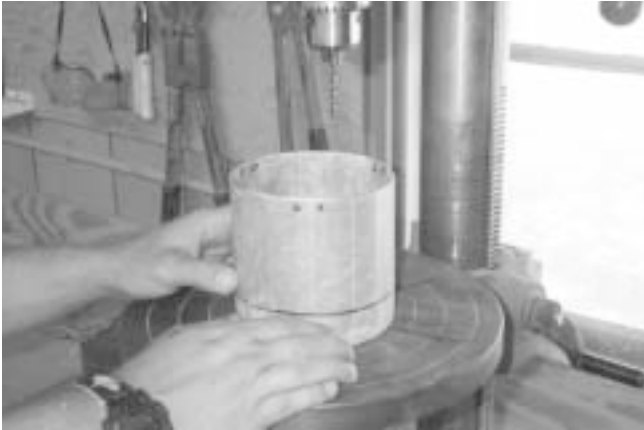
Figure A.7. Drill three equally spaced pairs of holes 1 cm from the top of the ring. Each hole should be 5 mm from its pair.
