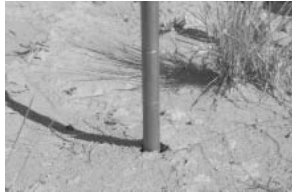
Figure 7.4. Record the number of strikes required to reach each 5 cm (2 in) increment (marked by the scribed marks on the rod).
