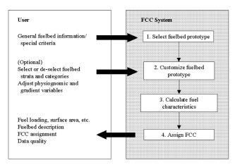
**Fig. 1.** User-provided general fuelbed information identifies a fuelbed prototype. The prototype identifies the kinds of fuel present (fuelbed strata and categories) and their qualitative (physiognomy) and quantitative (gradient variables) features. The user can then adjust the prototypic information. Next, the system calculates fuel properties and fire parameters based on the customized fuelbed data. Finally, the system assigns the fuelbed to a stylized Fuel Characteristic Class.
