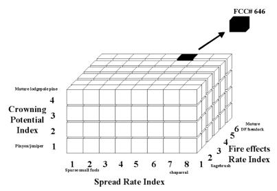
**Fig. 4.** 192 stylized fuel characteristic classes in 3-dimensional space grouped by three critical attributes of spread rate, crowning potential, and fire effects.
