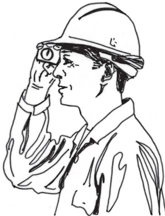
Figure 4-8. Estimating slope with a clinometer.
