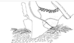
Figure FL-11. Use your boot to carefully pull the litter and duff layers away, until you are down to mineral soil.
