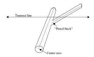
Figure 8. A piece of CWD crossed twice because it is branched. Treat as two separate pieces, with diameter measured at each point of intersection. Record the length of each piece separately.
