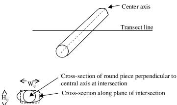
Figure 15. Overhead view of a CWD piece at a horizontal angle to the line transect.
