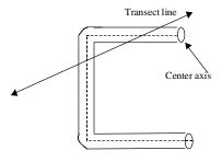
Figure 10. A U-shaped piece of CWD crossed twice by the transect line. Measure diameter at each point of intersection. Measure length once, but record each time the piece is crossed.
