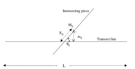
Figure 13. Measuring angle and length for an intersecting piece.
