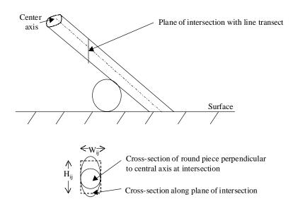
Figure 16. Side view of a CWD piece at a vertical angle to the line transect.
