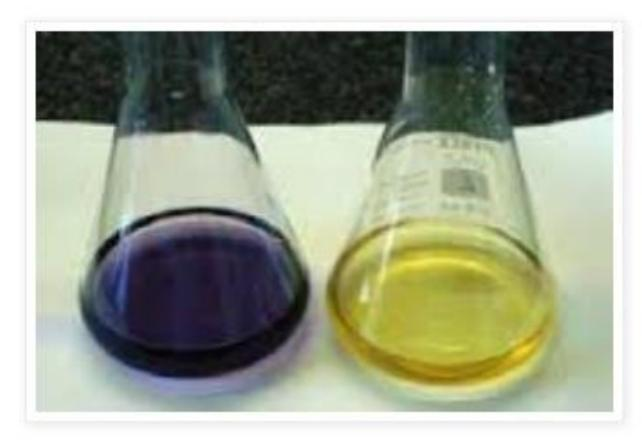
After solution reaches a pale yellow colour, a few drops of a freshly prepared starch solution are added. The solution becomes blue-black forming Starch-iodine complex and the titration is continued until it goes colorless.
