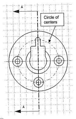
8) Dimension the 3 **Diameter Dimensions** shown in the figure. Notice that the dimensions do not look like the dimensions shown in the figure. Select all
