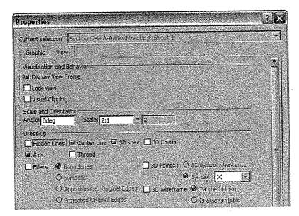
4) Change the properties of the cutting plane line. Right click on the cutting plane line and select **Properties**. In the *Properties* window, click on the **Call out** tab and set the line thickness to 3 and the line type to 5. Set the length of the arrow base to **0.001** mm. Set the arrow head type to solid, the length to 5
