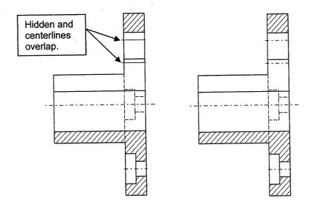
Section views usually do not contain hidden lines. Eliminate the hidden lines in the right side section view.
