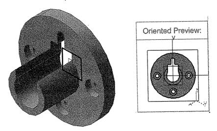
5) Your sheet should contain the front view and areas for the top, right and isometric views. These are not necessary in their final positions. The prompt line will read, *Click on the sheet to generate the view or redefine the view orientation using the arrows*. Look at the front view. If the orientation is not correct, you can use the blue circle with four arrows to reorient the front view. If the orientation is correct, click on the sheet.
