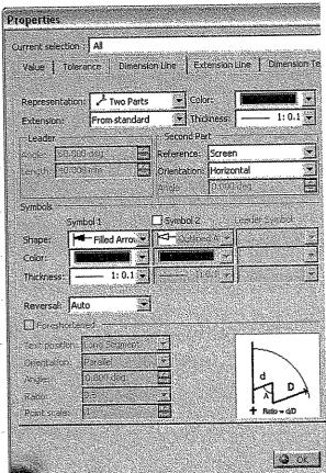
9) Notice that the dimension for the counterbored hole is not correctly stated. shows only the diameter of the counterbore. Access the Properties window for that dimension. Select the Value tab and activate the Fake Dimension toggle. Enter a Main Value: of 4 mm. This is the diameter of Select the hole. the Dimension Text tab. Enter 3X in the top box of the Main Value field. This indicates that there are 3 counterbored holes.
