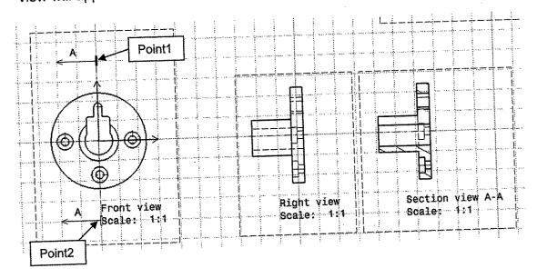
2) Change the look of the section lines. In the section view, double click on the section lines. In the *Properties* window click on the **Pattern** tab and change the angle to **45°** and the pitch to **1 mm**.
