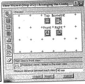
4) The prompt line will read, Select a reference plane on a 3D geometry. At the top pull down menu, select **Window** and then your part drawing. Move your mouse over the plane that is parallel with the back of the part. An Oriented Preview will appear in the corner showing you what the front view will look like. If this is acceptable, click on the plane.
