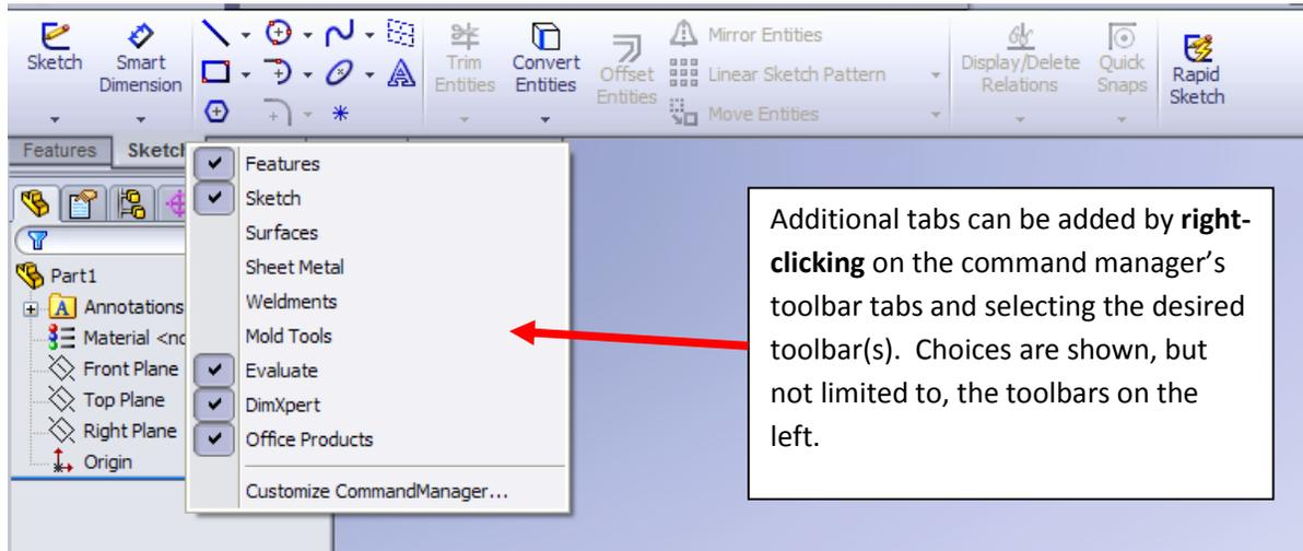
Additional tabs can be added by **right-clicking** on the command manager’s toolbar tabs and selecting the desired toolbar(s). Choices are shown, but not limited to, the toolbars on the left.
