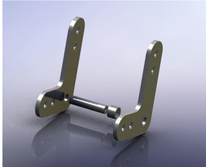
Figure 12: Bell crank design.
