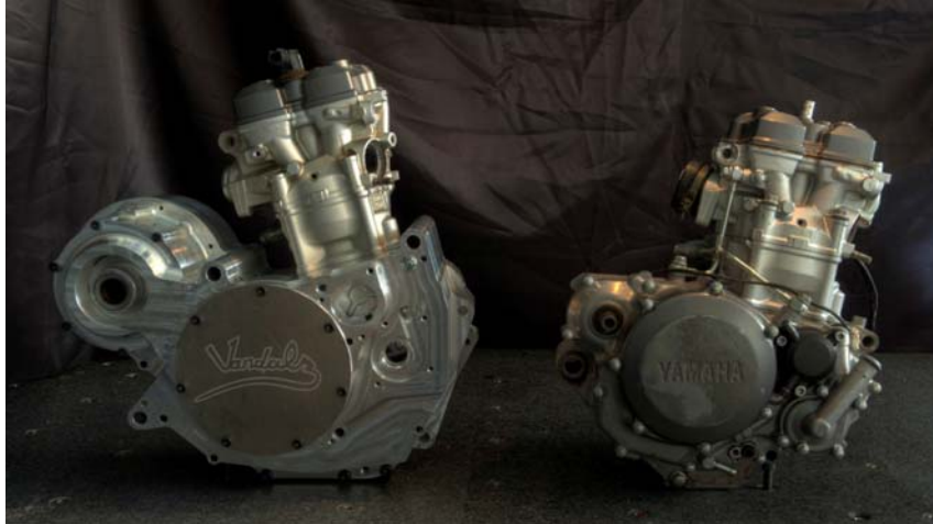
Figure 6: Cylinder Orientation Compared to a Stock Engine
