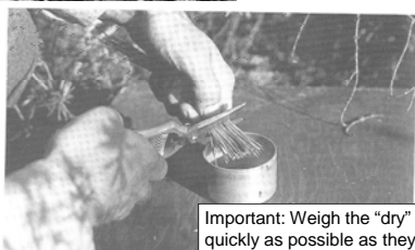
Figure 3.18. Fuel samples are clipped into a can, weighed, dried, and weighed again to determine moisture content. Photo by Melanie Miller. From Norum and Miller (1984).
