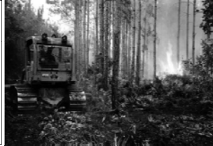
Dozer making a fire line – Florida, 1998 (FEMA)
