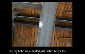
The top hobo was situated just inches below the underside of the bottom flange of the steel beam that spanned across the space.
