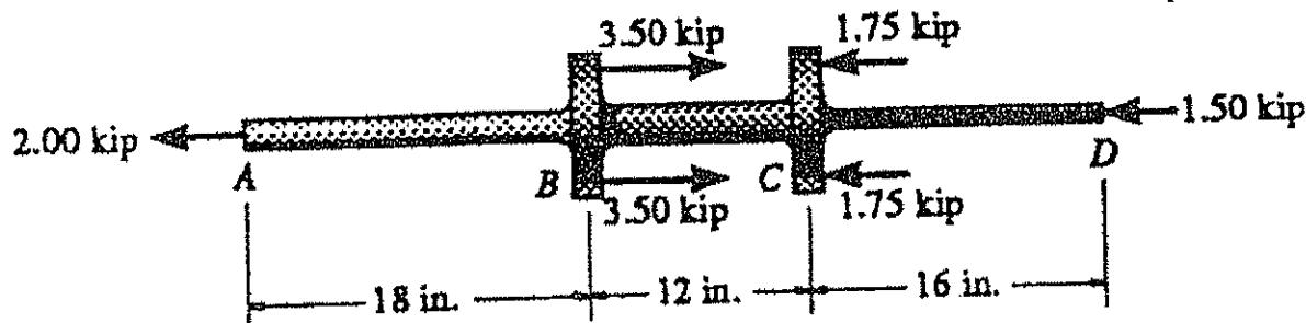
2) (25 pts.) A solid constant-diameter shaft is subjected to the torques shown in the figure. The bearings shown allow the shaft to turn freely.
