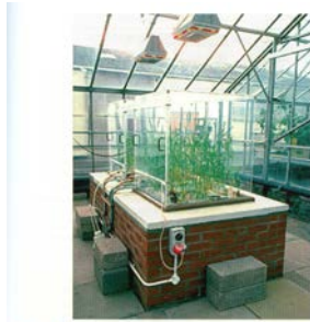
FIGURE 10.3 Laboratory and Greenhouse Experiments. Diffusers and enclosures may be used to maintain constant elevated \text{CO}_2 levels, whereas greenhouses or other warming devices may be used to manipulate temperature. Courtesy of SCF
