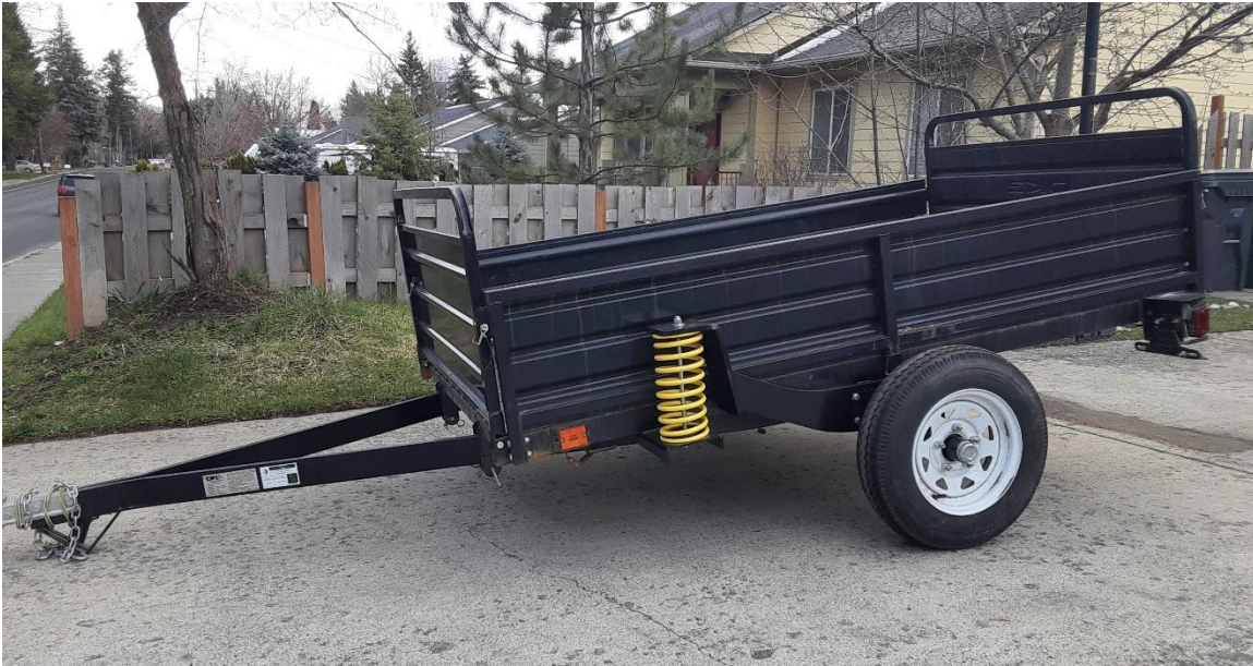
Figure 1. Single axle trailer with 3S suspension system.
