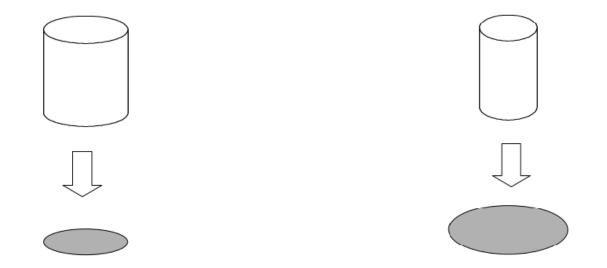
The shaft tolerance should be (-), in relation to the maximum shaft size, to prevent the shaft from being to large to fit the hole . The hole tolerance should be (+), in relation to the minimum shaft size, to prevent the hole from being to small for the shaft to fit.
