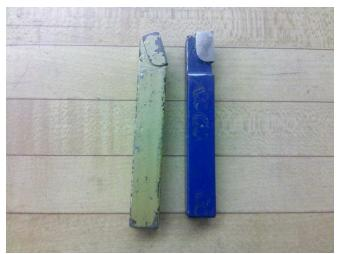
**Right Handed Cutting Tool** – The cutting edge is on the right side of the bit with clearances below the right cutting edge and the front. This bit is used for facing and shortening parts. No cutting oil is necessary with this tool. The speed follows the chart.
