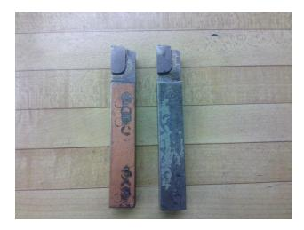
**Left Handed Cutting Tool** – The cutting edge is on the left side of the bit with clearances below the left cutting edge and the front. This bit is used for turning down outside diameters of parts. No cutting oil is necessary with this tool. The speed is determined by the chart in the shop.
