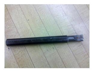
**Inside Threading Tool** – This tool is used to thread the inside of a part. As with the outside threads this is done when you don't have a large enough tap or the correct size. This process will be discussed in the Threading Section.
