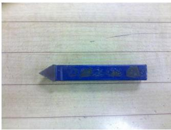
**Outside Threading Tool** – As the name implies this tool is used to cut outer threads in a part. This is usually done when you don't have a big enough or a specific die to thread the part. This operation will be discussed in the Threading Section.
