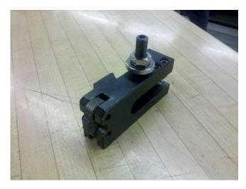
**Knurling Tool** – This tool is used to put a knurl on a part. This improves the grip of the part. To knurl a part, touch up to the surface and dial in the X-direction .050 in and move the tool in the Z-direction for the desired knurl. Run the lathe at 100 rpms.
