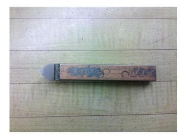
**Chamfer Tool/Two-Sided Cutter** – The chamfer tool, usually cut at 90° is used to create chamfers at this angle. The bit can also cut in either direction.
