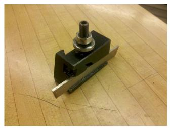
**Parting Tool** – The parting tool is a piece of flat steel with clearance under the cutting edge. It is used to cut the part at the desired location. Cutting oil must be used or the part will bite. The speed is half of the chart speed.
