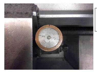
This the dial to use for threading. Engage when the desired dash mark is straight up.
