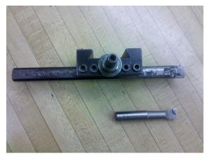
**Boring Bar** – This tool is used to bore holes into parts. It is easiest to drill a hole and use a small boring bar. From here you can work up to a larger boring bar. Do not use cutting oil and follow the chart for speed.
