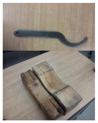
The wrench and blocks used to change the chucks. The small block on the left is for the 4-Jaw and the larger one on the right is for the 3-Jaw.
