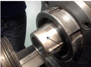
This picture shows the key that it is necessary to line up when connecting the chuck to the machine.
