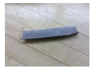
High strength steel is very useful in tool grinding. You can make tools to do many different operations. If one of the basic tools doesn't work for the desired operation you can take a HSS tool blank and shape a tool for the necessary application. Take the tool to the grinding wheel and use the knowledge you have gained on the lathe about tool clearances to create your tool.
