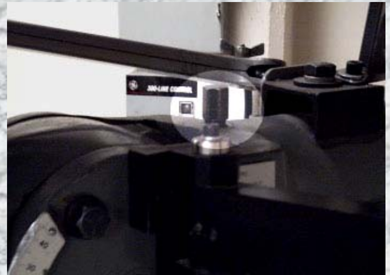
Figure 2 Adjusting bolt for X-axis tramming
