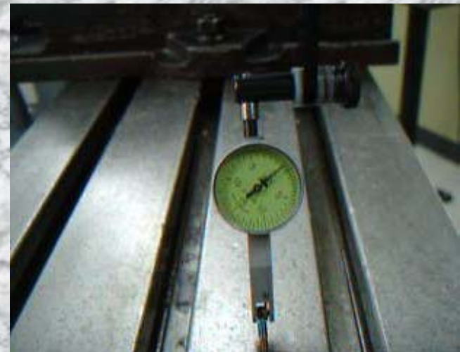
Figure 4 Dial indicator installed on chuck
