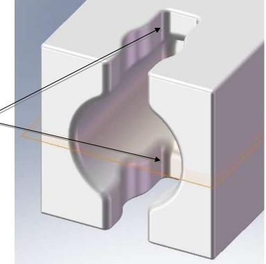
If strength is not a concern, consider instead where support material will be placed. Choose an orientation that will put support material around external features instead of internal features such as holes or slots. Not only is the support material much more difficult to remove on internal features, but often the attempt to remove it can cause the part to split apart at a layer transition surrounding the internal feature.
