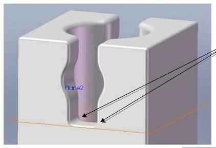
These stress concentrations cross a layer transition (layer orientation is represented by the plane). The top two flanges will break off at this transition if any forces are applied in the slot.
