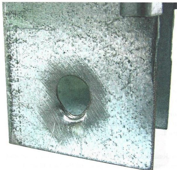
FIGURE 1.6 Bearing stress failure at a bolted connection.
