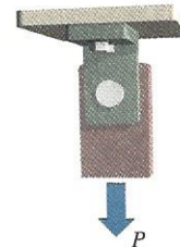
FIGURE 1.2a Single-shear pin connection.
