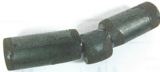
FIGURE 1.4 Double-shear failure in a pin specimen.
