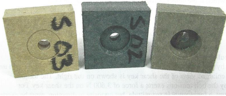
FIGURE 1.5 Punching shear failure in composite wood block specimens.
