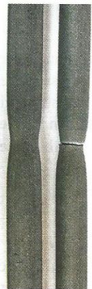
FIGURE 3.11 Necking in a ductile metal specimen.
