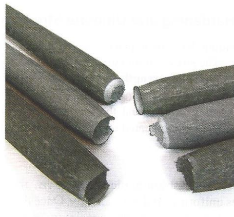
FIGURE 3.12 Cup-and-cone failure surfaces.
