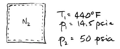
GIVEN: Nitrogen in a closed, rigid tank
