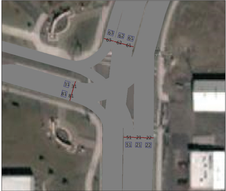
Figure 106. Signal head and detector numbering example
