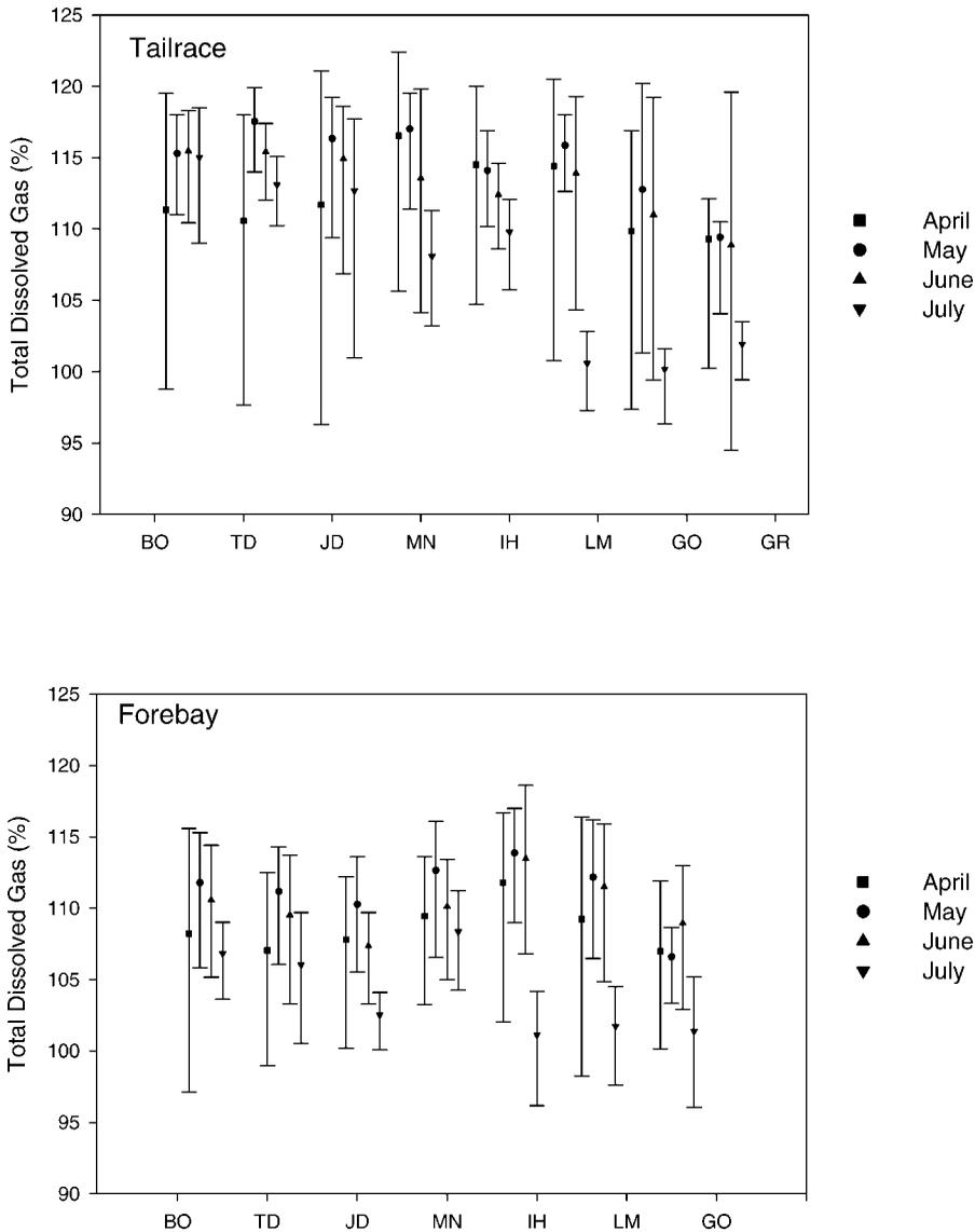
FIGURE 2.—Mean and 90th percentiles of hourly total dissolved gas concentrations in the lower Columbia and Snake River dam tailraces and forebays, April–July 2000. Abbreviations are as follows: BO = Bonneville Dam, TD = the Dalles Dam, MN = McNary Dam, IH = Ice Harbor Dam, LM = Lower Monumental Dam, GO = Little Goose Dam, GR = Lower Granite Dam. Data are from the U.S. Army Corps of Engineers, 1998.
