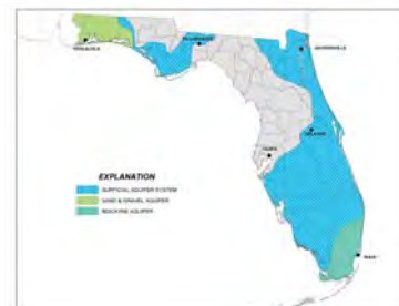
This map shows where the Surficial Aquifer Systems in Florida are found at the land surface. This is where these sources of drinking water are at their most vulnerable.
