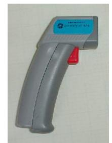
Your instrument of choice for this exercise is the Raytek Hand-Held Infrared Thermometer MT-4—a device for measuring surface temperatures. This pyranometer measures the long-wave infrared radiation emitted by a surface. It then calculates the temperature of the emitting surface using a fixed emissivity value (~0.85, typical of non-metallic surfaces). It has a nifty integrated laser pointer to indicate the spot being measured.
